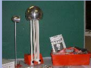
Van De Graaf generator (P015) and Primary electricity kit (P001)
